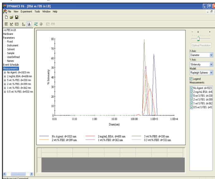
Figure 2. TiO<sub>2</sub> particle size distribution in LB calculated by the built-in regularization algorithm shows the effect of BSA and FBS dispersing agents. The corresponding hydrodynamic diameter (*d*) of TiO<sub>2</sub> was determined to be 1023 nm, 608 nm, 330 nm, 399 nm, 362 nm, and 532 nm for no dispersing agent, 2 mg/mL BSA, 5 wt.% FBS, 2 wt.% FBS, 1 wt.% FBS, and 0.5 wt.% FBS, respectively.
