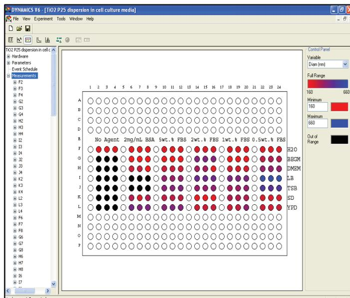
Figure 1. Spectra view of TiO<sub>2</sub> nanoparticle dispersion in water and six different cell culture media (BEGM, DMEM, LB, TSB, SD, and YPD) suggests severe agglomeration in all media without dispersing agents, improved dispersion in most media using 2 mg/mL BSA, and the best dispersion using ≥1 wt.% FBS.
