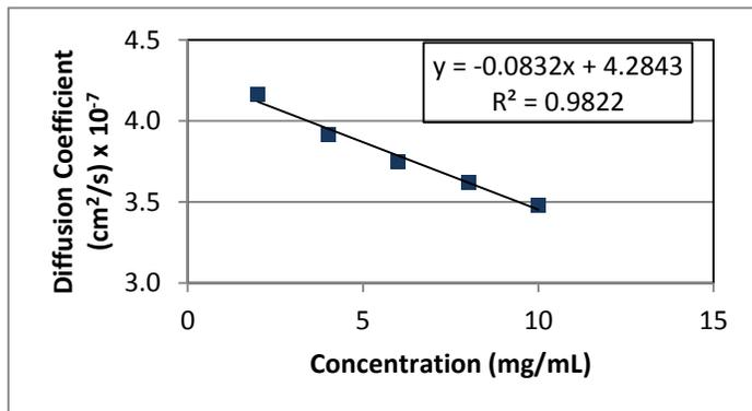
Figure 3. Diffusion coefficient as a function of concentration for Protein 1. The slope divided by the y-intercept yields a  $k_D$  value of  $-1.9 \times 10^{-2}$  ml/mg.
