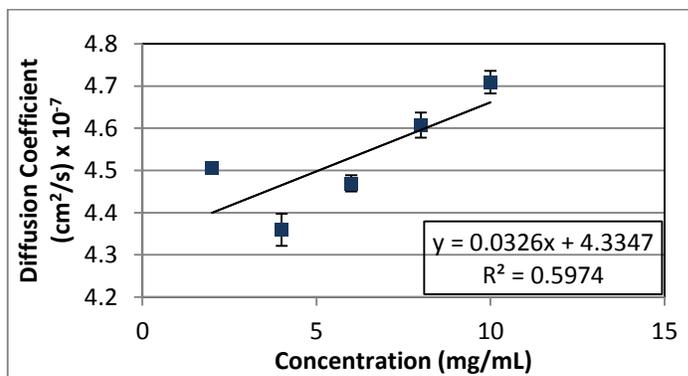
Figure 4. Diffusion coefficient as a function of concentration for Protein 2. The slope divided by the y-intercept yields a  $k_D$  value of  $7.5 \times 10^{-2}$  ml/mg.
